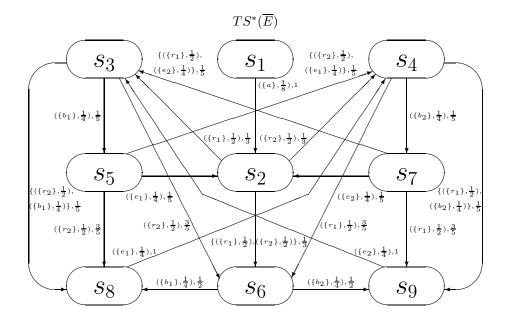
Figure 25: The transition system without empty loops of the shared memory system
