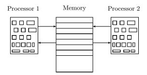
Figure 24: The diagram of the shared memory system
